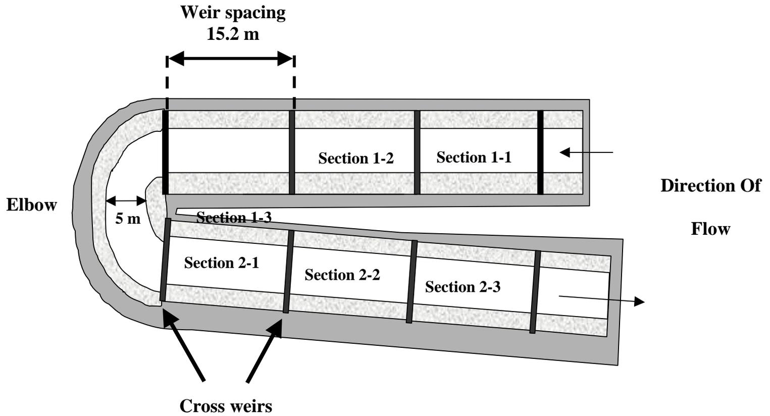
Figure 1. The dimensions of the artificial stream located at the Cle Elum Supplementation Research Facility that was used to evaluate the breeding success of female spring Chinook salmon. Not drawn to scale.
